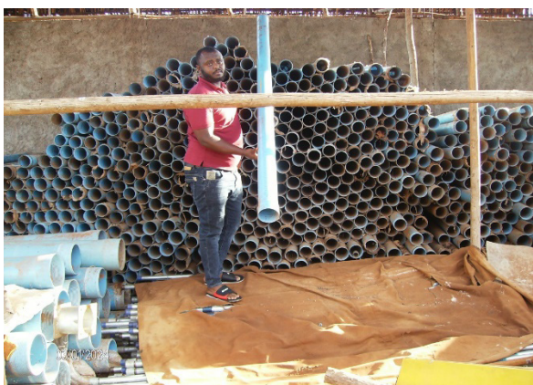
A 4-inch PVC casing is the most common material used for community wells with hand pumps.
