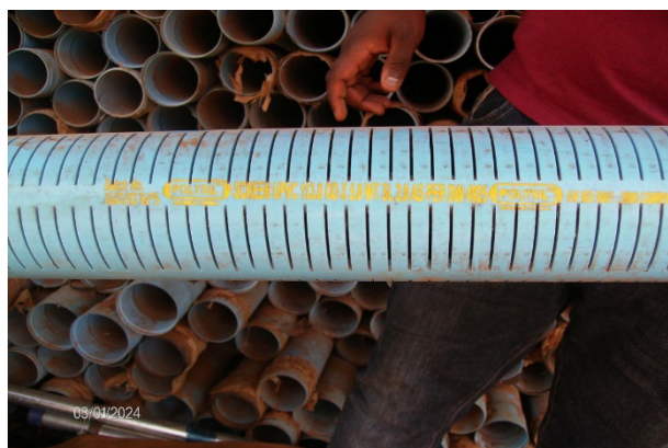
The PVC casing is slotted in the aquifer layer for groundwater collection.
