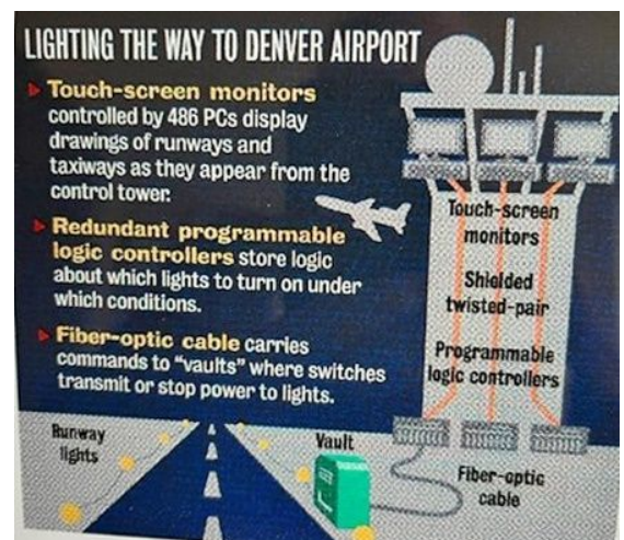
DIA touch screen lighting control system schematic.
