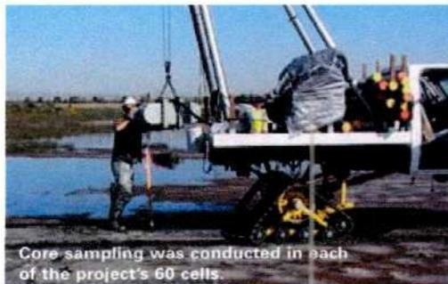
Core sampling was conducted in each of the project's 60 cells.
