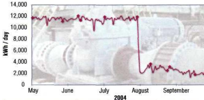
Average energy consumption at the Nukus pump station was about 11,500 kilowatts a day prior to the system overhaul. After the new system startup in August, daily energy consumption dropped five times to about 2,300 kilowatts.
