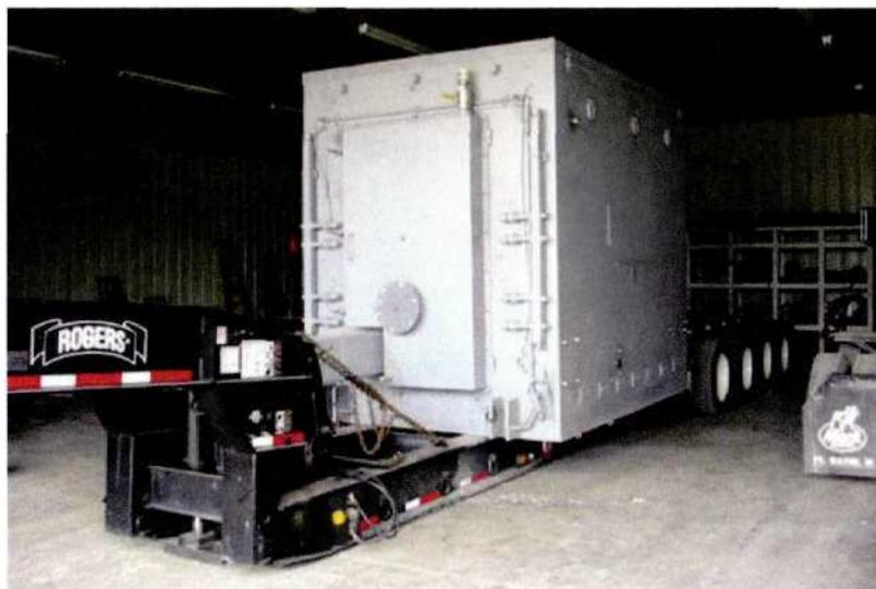
The Donovan Blast Chamber, used to destroy unexploded ordnance and obsolete munitions, is being modified in a collaborative effort by several CH2M HILL companies to safely explode chemical weapons. The latest advancement in the technology is currently being tested and is expected to be completed by next spring.
