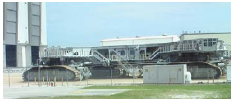
The crawler that carries the 6 million ton shuttle and booster rocket. Each tread cleat weighs 1-ton!
