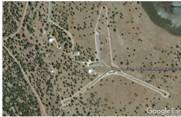
The NPOI has 9 fixed telescope positions on each of 3 arms 120° apart and 250 meters long.
