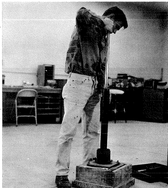
Compaction Test. To determine maximum density and optimum moisture content of soil materials under standard conditions.
