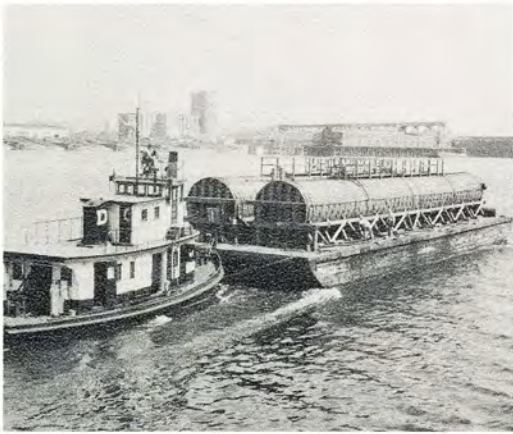
The summertime disposal problem for the Publishers' Paper Company, Oregon City, Oregon, is handled by barging the sulphite liquor to the Columbia River.
